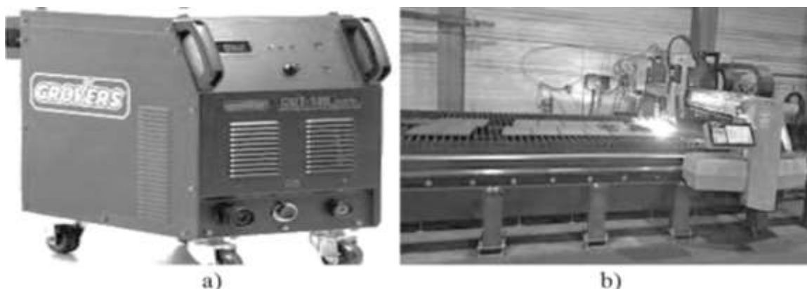
5.8-rasm. Detallarga plazma usulida ishlov beruvchi plazmatron (a) va plazma usulida metallarni kesish (b) jarayonlari.
